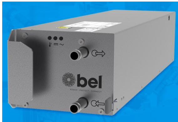
Figure. The TLP5000-1048 is a 5-kW, three-phase ac-dc converter with adjustable dc output. Liquid cooling (no fan) makes this power supply suitable for a wide variety of high power industrial applications. This power supply has been designed with emphasis on reliability and long life. Parallel operation is possible for up to 12 units (up to 60 kW).
