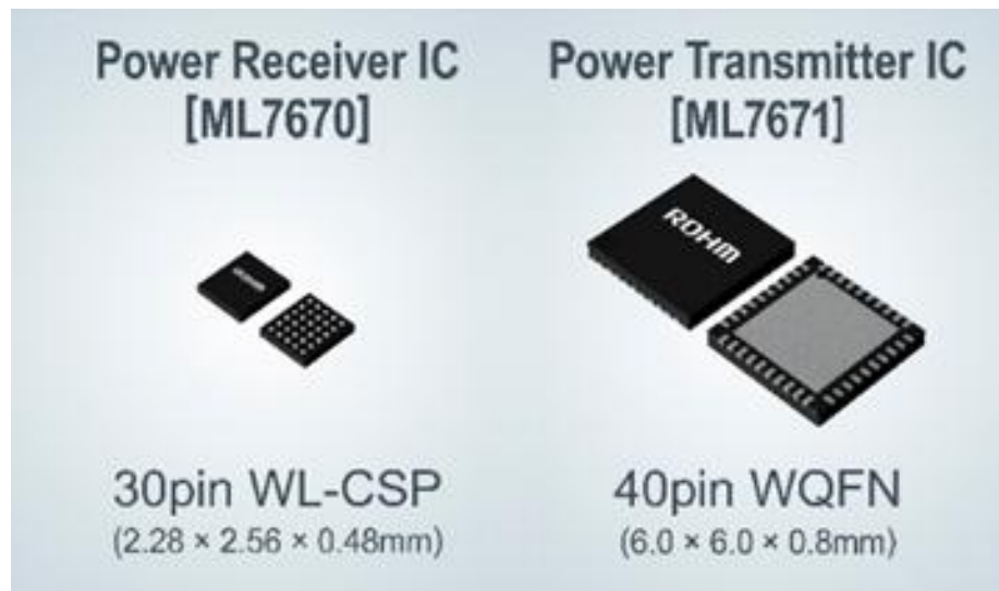
Fig. 1. The ML7670 power receiver IC achieves a maximum power transfer efficiency of 45% in the 250-mW low output range—all in what's described as an industry-leading form factor of just 2.28 \times 2.56 \times 0.48 mm. According to the vendor, a key feature of the chipset is superior performance that surpasses the efficiency of comparable products in the same class by optimizing elements such as coil matching, rectifier circuitry, and reduced losses in switching devices. What's more, all firmware required for wireless power delivery is embedded directly within the IC, eliminating the need for a host MCU. This significantly reduces board space along with development workload in device design.
