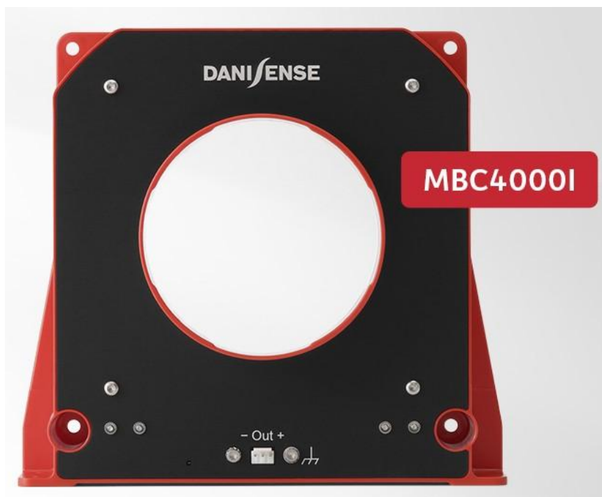
Figure. The MBC4000I, a new fluxgate generation ac-dc current transducer, offers high-precision current measurements of up to 4000 A and more with accuracy up to 10 times higher than a traditional Hall-effect transducer. Measurement error is below 0.05% over temperature from -20°C up to +85°C. It also offers ultra-low sensitivity drift and a large Ø121-mm aperture for busbar applications.
