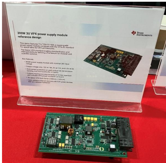
Fig. 2. The TIDA011004 reference design is a space-grade power supply module compliant with the VITA-62 standard for space-rated 3U VPX architectures. The eval board and block diagram are shown here.
