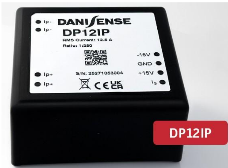
Figure. With its 32-mm high, 250-g PCB-mount package, the DP12IP series current transducer features a maximum linearity error of just 10 ppm and supports current measurement up to 18 A.
