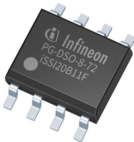
Fig. 1 Alternatives to photovoltaic isolators (PVI), photovoltaic relays (PVRs), and electromechanical relays (EMRs), Infineon's iSSI20B02F, iSSI20B03F and iSSI20B11 coreless-transformer solid-state isolators provide powerful energy transmission over a galvanic isolation barrier to drive the gates of MOS-controlled power transistors, such as CoolMOS, OptiMOS, or TRENCHSTOP IGBT. The output side of the isolators does not require a dedicated voltage supply to drive the power transistor's gate and offers advanced control functions such as fast turn-on, fast turn-off, overcurrent protection and overtemperature protection.
