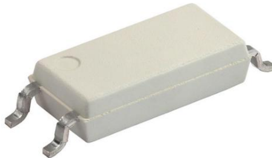
Figure. The optocoupler's ability to isolate dc voltages up to 1000 V enables its use in next-generation high-voltage EV architectures. It consists of an infrared emitting diode, optically coupled to a silicon planar phototransistor detector in a low-profile LSOP package with creepage and clearance distances of \geq 8 mm.
