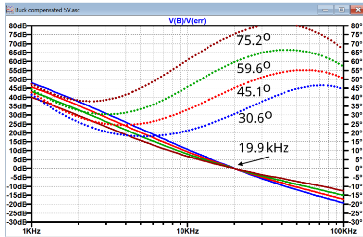
Fig. 2. Bode plots of the simulated buck converter.
