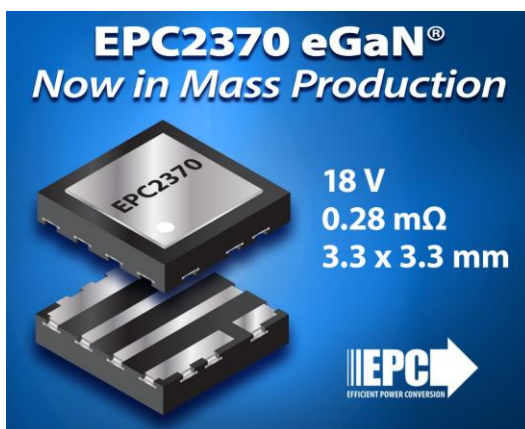
Figure. Featuring an R_{DS(ON)} of only 0.28 m \Omega and a transient voltage rating of 22 V, the EPC2370 eGaN FET enables high-efficiency, 1-MHz or higher switching, and increased power density for advanced high-current dc-dc converters.
