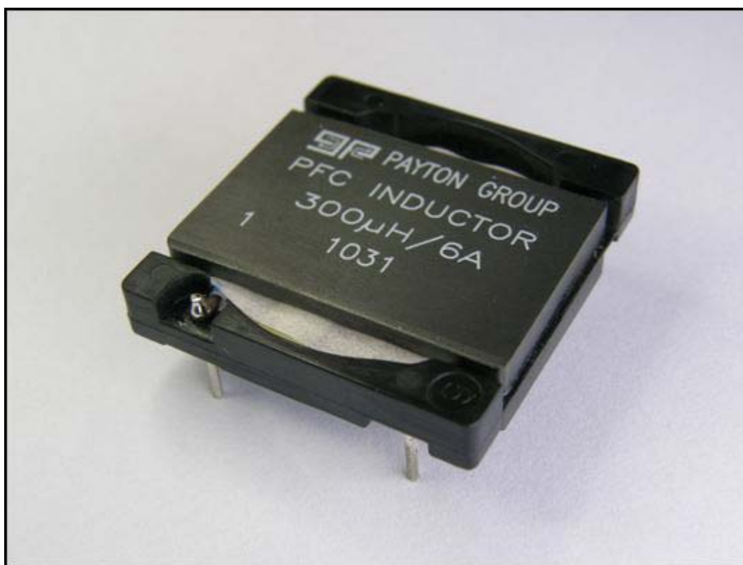
Figure. This 8-mm high planar inductor enables the development of 200-W power supplies with a profile of less than 1 cm as required in large-format LED televisions.
